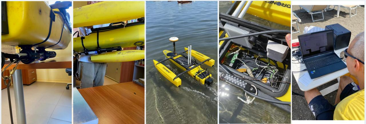
we have equipped the Tridrone with new i7 PC, Hypack Environmental mapping, an EXO1s multiparametric probe and telemetry. All powered by the Tridrone's battery.
