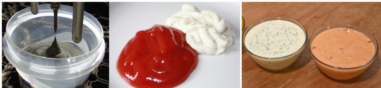
Figure 6: Consistency of fluid mud, ketchup/mayonnaise, and salad dressings at the 2 Pa*s level
