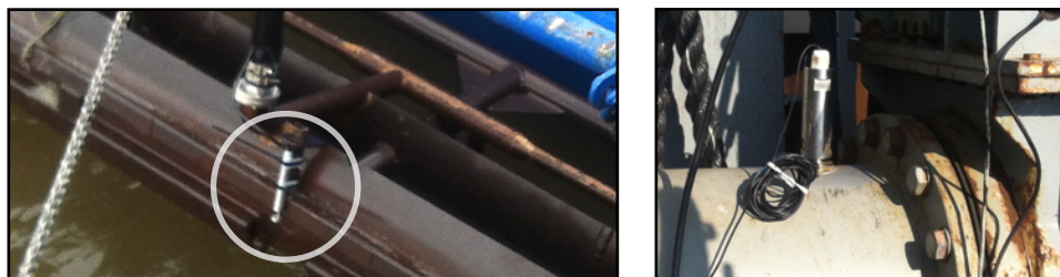
Figure 12: Density probes mounted on the bed leveller frame and at the suction pipe of the cutter dredger
