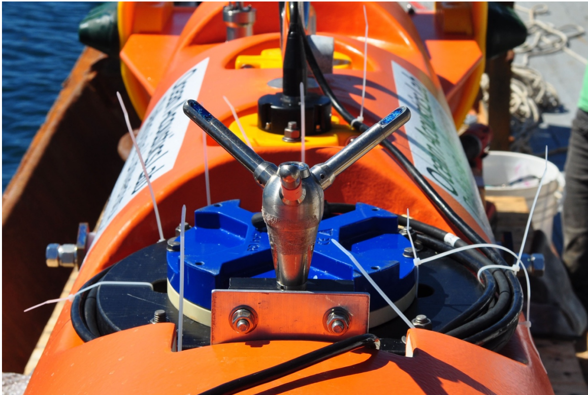
Figure 2: ADV integrated into the Nemo moored platform.
