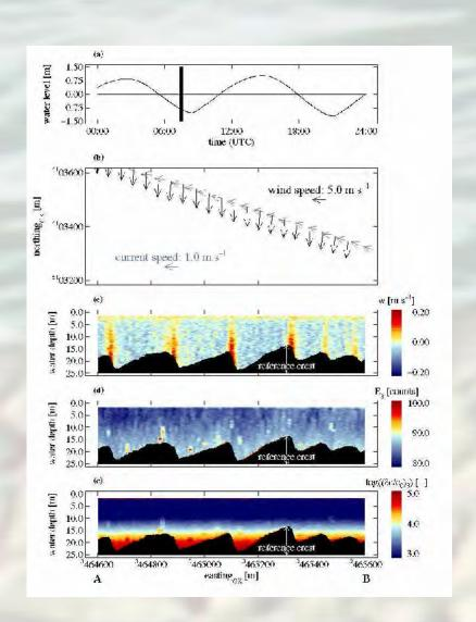
Three dimensional presentation of w and  $E_3$  (color coded) as a function of water depth of run 51 along transect AB as shown on the left side
