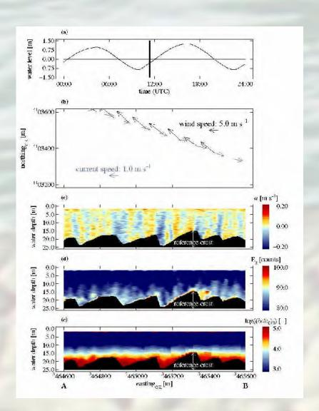
Three dimensional presentation of w and  $E_3$  (color coded) as a function of water depth of run 64 along transect AB as shown on the left side
