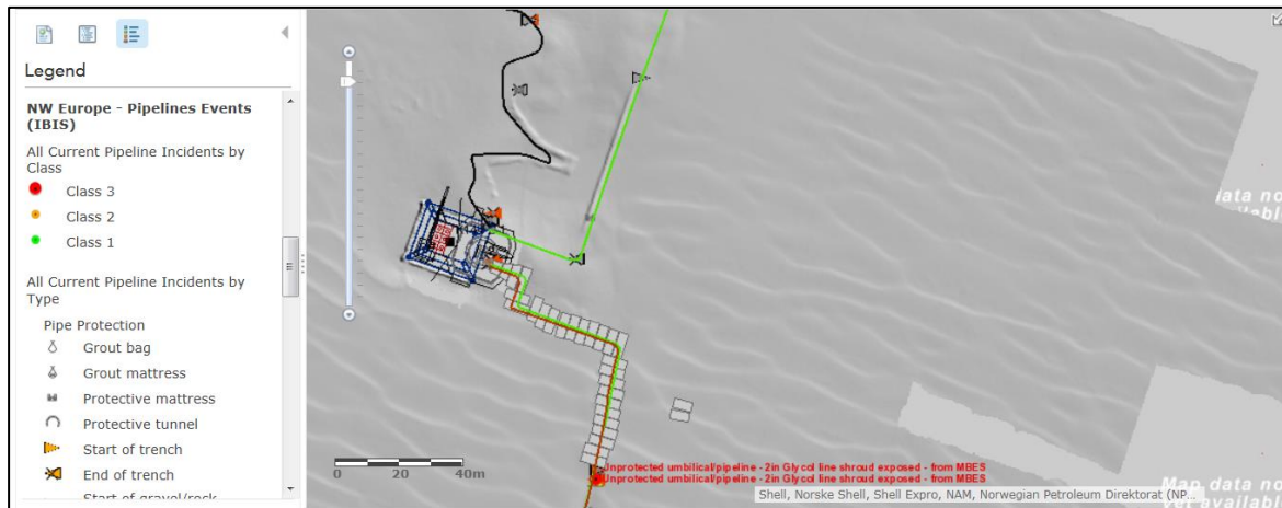
Figure 5: Example of pipeline inspection data in a corporate web map.
